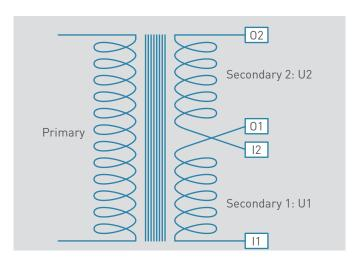
The secondary voltages U1 and U2 should be the same for parallel connection.
