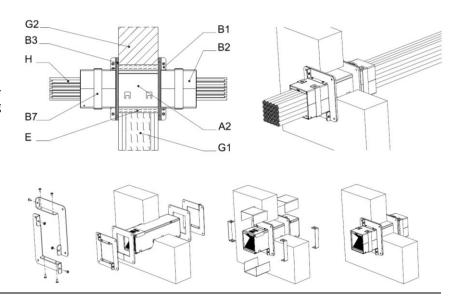
Single EZ-Path® Pathway Series 44+ secured to rigid or flexible wall using plate kit EZP144WT
