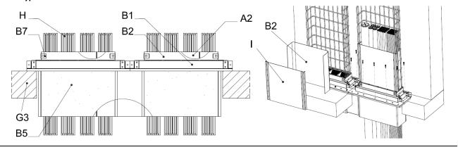
Single up to five EZ-Path® Pathways Series 44+ secured to rigid floor using plate kit EZP544MBE in association with one min 50mm thick Rockwool Firepro® Ablative Coated Batt and min 100mm thickness of Rockwool FirePro® Firestop Compound.
