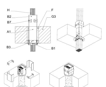
Single EZ-Path® Pathway Series 44+ secured to rigid floor using plate kit EZP144MBE. Annular space filled with regular construction mortar.
