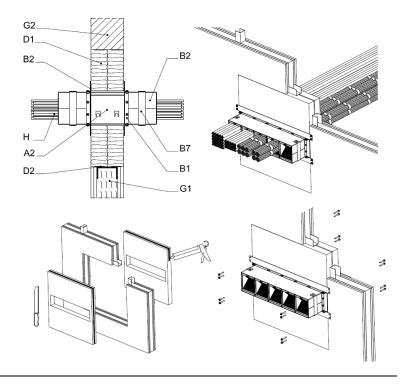
Single up to ten EZ-Path® Pathways Series 44+ secured to rigid or flexible wall using plate kit EZP544WE in association with two STI SpecSeal® Composite Sheets installed on both sides of wall. Space between composite sheets filled with mineral wool batt insulation. Please refer to the Annex B "Resistance to Fire Classification".
