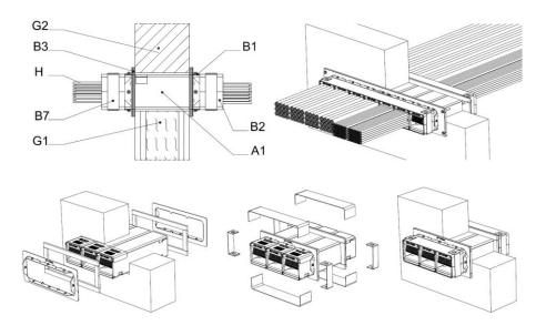
Single up to five ganged EZ-Path® Pathways Series 44+ grouted in rigid wall using regular construction mortar to fill annular space.
