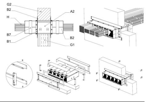
Single up to five EZ-Path® Pathways Series 44+ secured to rigid or flexible wall using plate kit EZP544WT
