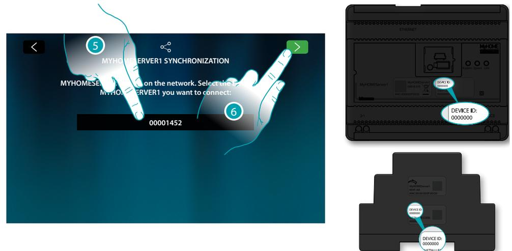
5. Select your MyHOMEserver1 identifying it by means of the ID DEVICE on the front or side of the device
