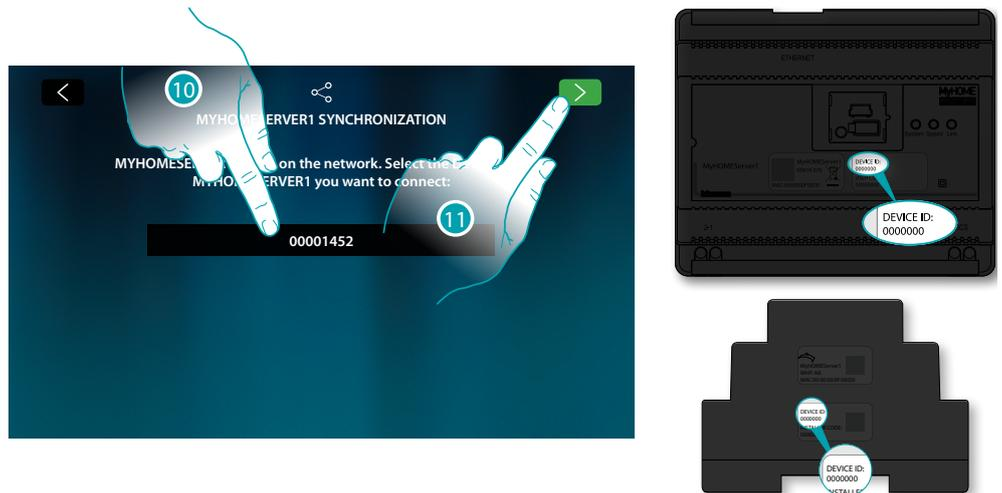
10. Select your MyHOMEserver1 identifying it by means of the ID DEVICE on the front or side of the device
