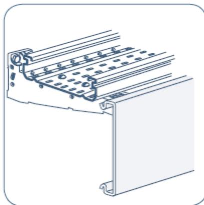
For easier installation, the cover can be simply hooked on the bracket during maintenance operations
