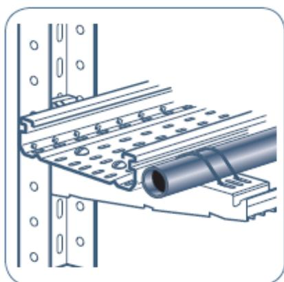
Special holes have been designed for fitting clamps so that pipes can be fixed on the bracket
