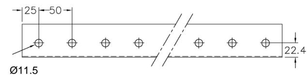
To fix pendant channels with ceiling brackets, use the nut and bolts M8x20
