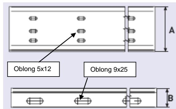
Slots 9x25mm in base of divider allow fixing with M8 screws
