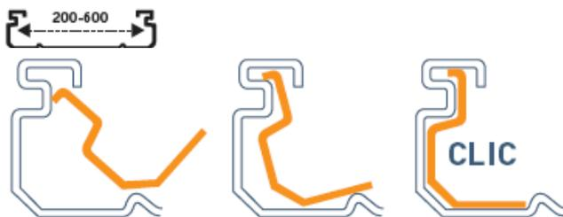
Marking system for installing couplers according to temperature conditions (20, 40 or 60°C) to enable the PVC to expand.
