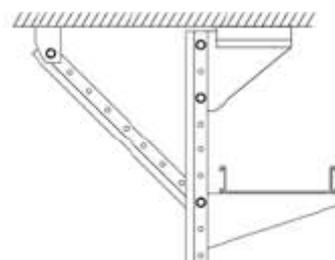
Reinforced installation (ceiling brackets + 1 pendant channel PVC), safe working loads max 310 daN
