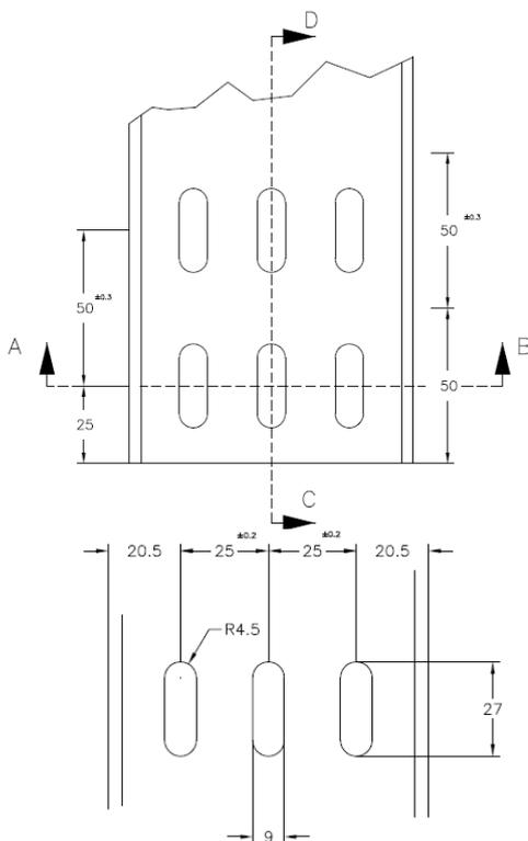
To fix pendant channels with ceiling brackets, use the nut and bolts M8x20
