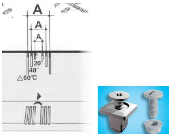
To lock with rapid fix rivet or bolt and nuts
