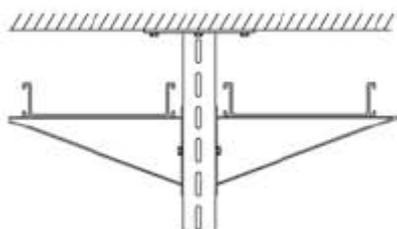
If more than 67 daN must be supported, the load must be evenly distributed to both sides of the pendant.
