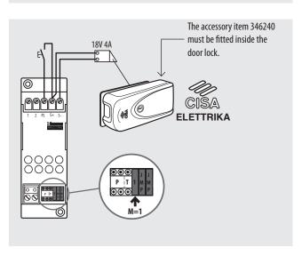
Wiring diagram - with auxiliary transformer
