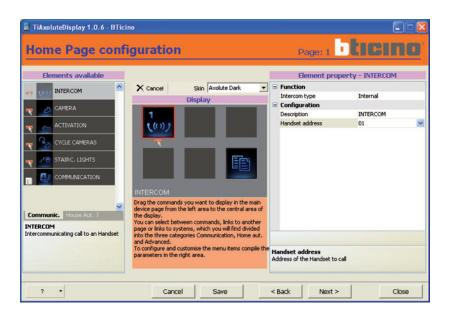
In the Element parameters area configure the address of the Handset to which the call refers and if you want customise the description.
