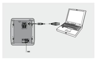
To ensure that the communication is successful, AXOLUTE VIDEO DISPLAY must be powered and not physically configured.
