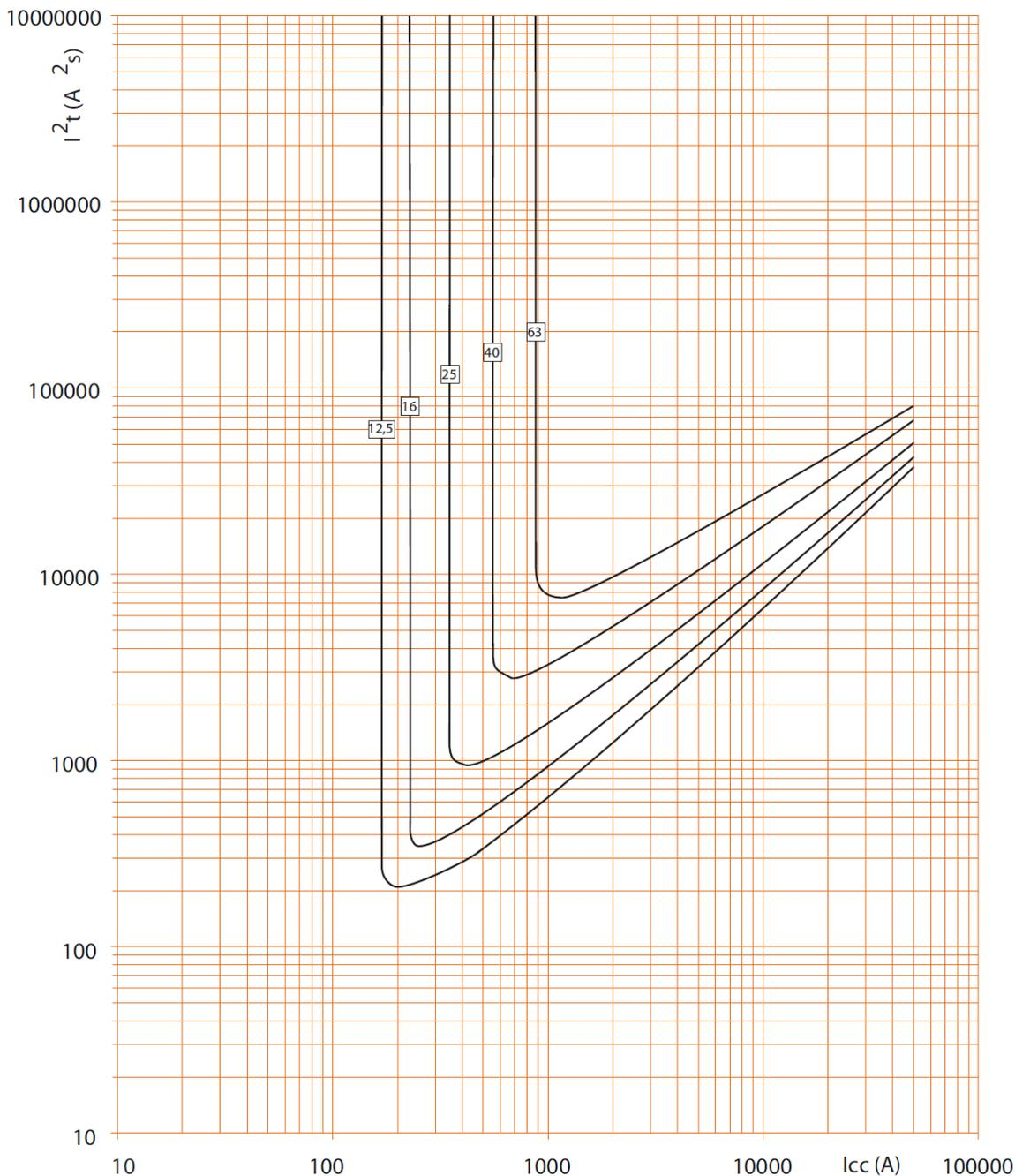
. Icc = Square value of symmetric component of the short circuit current ( kA ).
