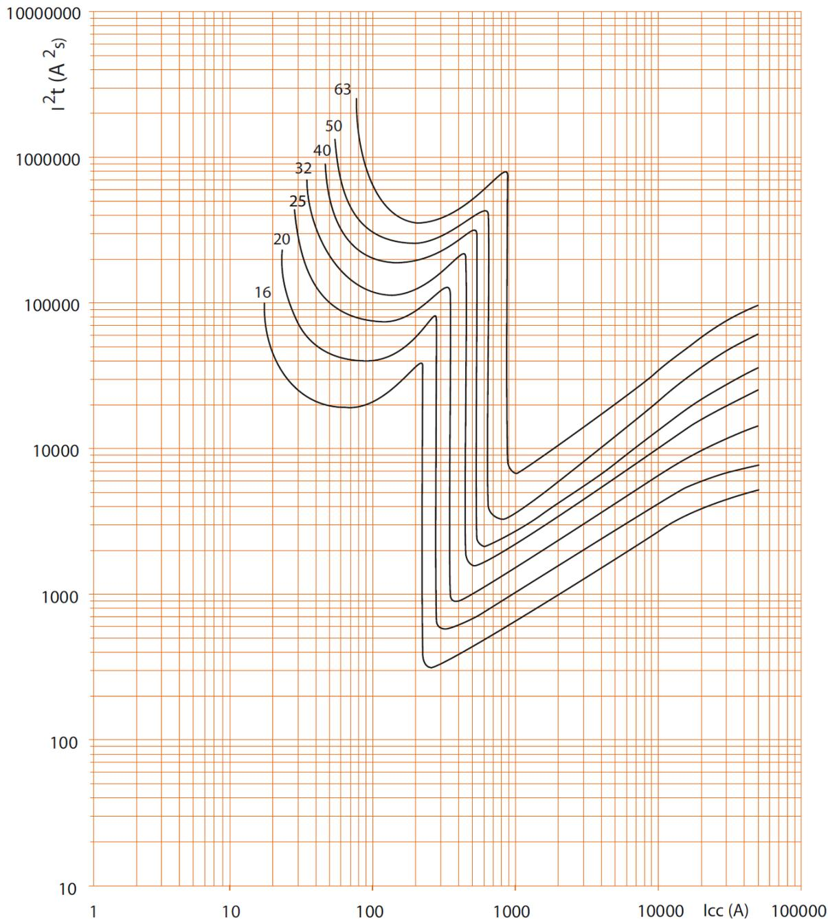
.  $I_{cc}$  = Square value of symmetric component of the short circuit current ( kA ).
